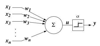
In this case, the output is given by y = 1 if  $u > \theta$  and y = 0 otherwise, where  $\theta$  is the threshold voltage of the neuron, and  $u = \sum_{i}^{n} w_i x_i$ .
