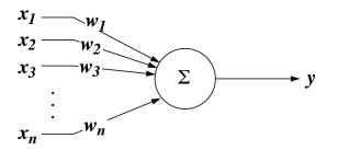
Each input wisis multiplied by a corresponding weight wi and these values are summed together to form the output y. Thus, the output is given as a function of the inputs and weights by the equation
