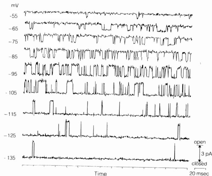
FIGURE 4.7 Current through nerve membrane as a function of time, for several membrane voltages. Upward steps are due to formation of sodium channels, downward steps are due to the channels' disappearance. The height of a single step is the current in a single channel, which increases approximately linearly with applied voltage, measured with respect to the sodium resting potential
