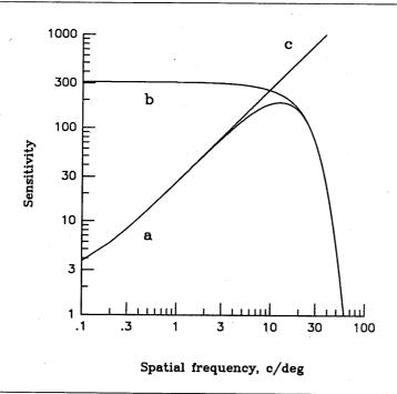
Figure 3: Curve a is the predicted retinal filter from equation 2.7 for a typical set of parameters, while curve b is  $R(f)^{-1/2}$ , which is the pure whitening filter. Finally, curve c is the low-pass filter d. The figure shows that at low frequencies curves d and d coincide and thus the system is whitening, while at high frequencies curves d and d coincide and thus the retinal filter is determined by the low-pass filter.
