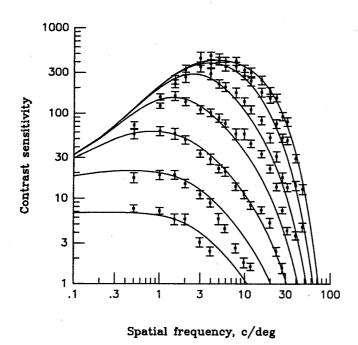
Figure 4: The family of solid curves are the predicted retinal filters (equation 2.7) at different  $I_0$  separated by one log units, assuming that the dominant source of input noise is quantum noise ( $N^2 \sim I_0$ ). No other parameters depend on  $I_0$ . The fixed parameters are  $f_c = 22$  c/deg,  $\alpha = 1.4$ ,  $\rho = 2.7 \times 10^5$ , N' = 1.0. The data are from human psychophysical contrast sensitivity measurements of Van Ness and Bouman (1967).
