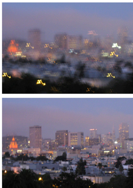
Fig. 1. (Upper) Camera shake during exposure creates image blur. (Lower) The same scene captured with the same exposure duration and a similar degree of camera shake but with an image stabilization mechanism (Canon PowerShot SD700 IS) that compensates for camera movement. How the visual system compensates for retinal image motion so as to prevent detail from being similarly corrupted by temporal integration processes in the brain is currently unknown.
