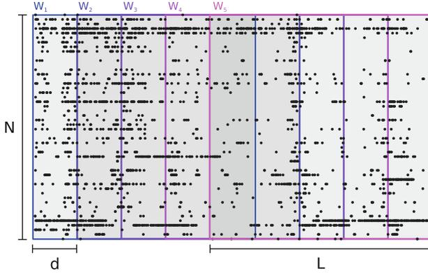
**Fig. 2. Windowing of binned neural activity.** To generate training data for the Hopfield network, spiking data of  $N$  cells are first binned and then training vectors are extracted using a sliding window. Windows of length  $L$  are shifted by  $d$  bins (here, we take  $d = 1$ ) resulting in training vectors of dimension  $n = NL$ . The above illustration shows five overlapping windows.
