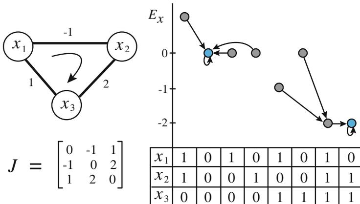
**Fig. 1. Small Hopfield network.** A 3-node Hopfield network with coupling matrix  $J$  and zero threshold vector  $\theta$ . A state vector  $\mathbf{x} = (x_1, x_2, x_3)$  has energy  $E_{\mathbf{x}}$  as labeled on the  $y$ -axis of the diagram. Arrows represent one iteration of the network dynamics; i.e.  $x_1$ ,  $x_2$ , and  $x_3$  are updated by Eq. (3) in the order of the clockwise arrow. Resulting fixed-points  $\mathbf{x}^*$  are indicated by blue circles (Color figure online).
